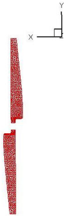
Figure 1: Unstructured surface mesh on a two-blade rotor.
